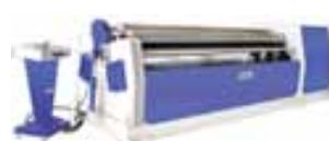
3-Roller Bender (For Curve Bending of Bull Nose and Pillar Wraps)
